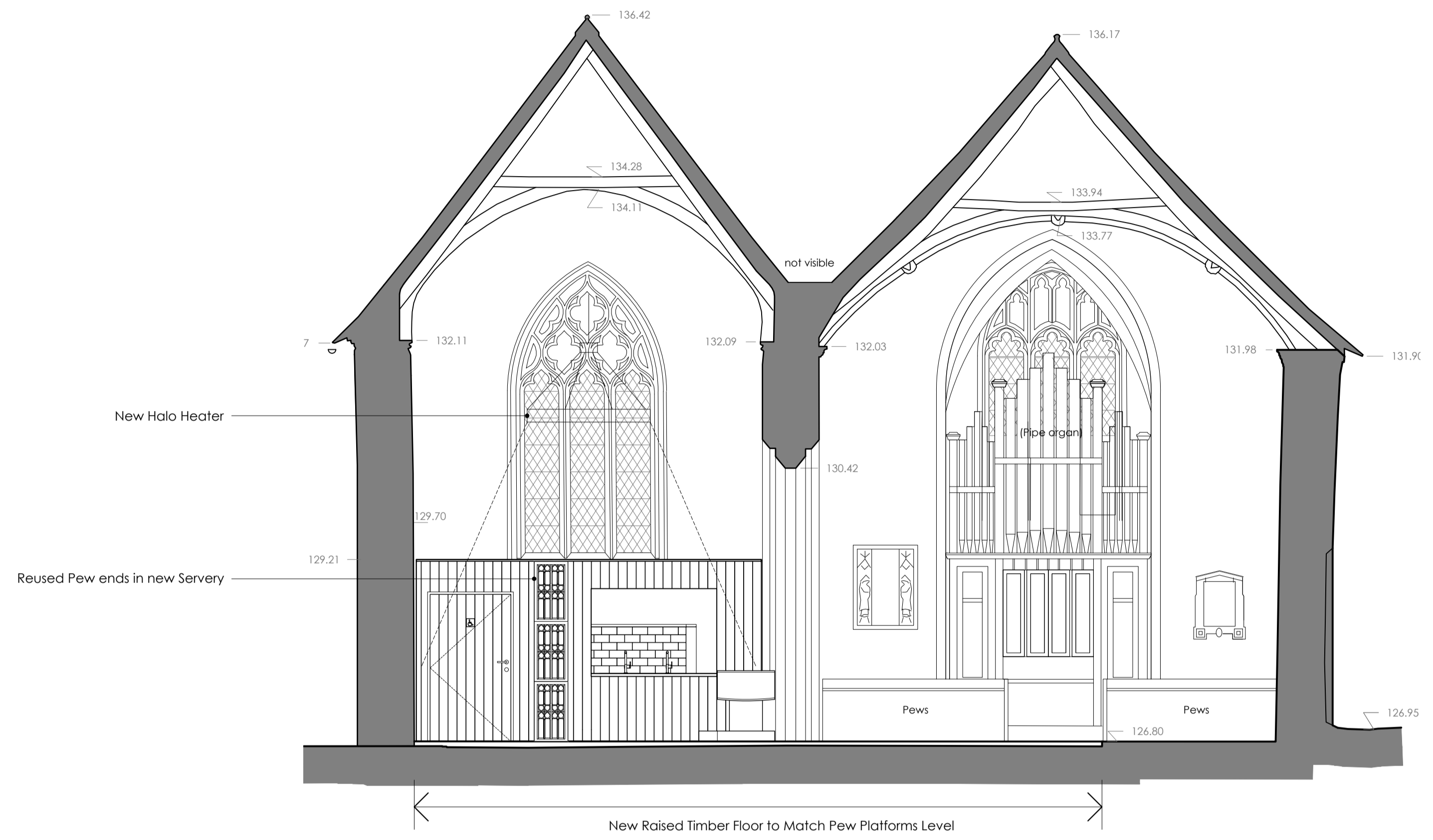
WC and Servery East Elevation
